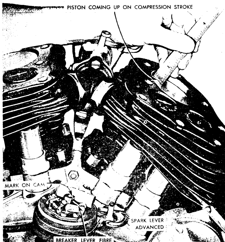
ILLUS. 72 TIMING IGNITION BY PISTON POSITION
