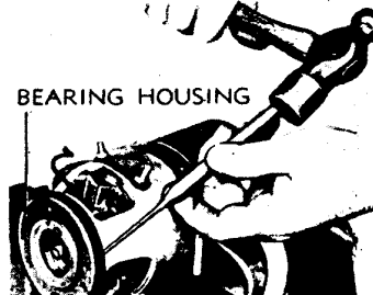
D—REMOVE BEARING HOUSING WITH DRIFT OR PULLER.
